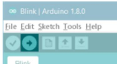
Wait a few seconds - you should see the RX and TX LEDs on the Arduino board flashing. If the upload is successful, the message "Done uploading." will appear in the status bar.
