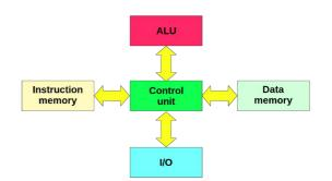
This has separate memory addresses for instructions and data meaning it can run a program and access data simultaneously.
