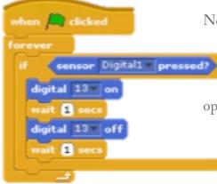
Now that the group have achieved an understanding of how the Arduino works, test this by asking them to use the button on their board to control the flashing LED. The button is plugged into Digital 1 so they should use the block that is an "IF" statement. Enable the group an opportunity to try this out, followed by the solution on the left.
