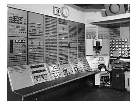
MIT introduces the Whirlwind machine on March 8, 1955, a revolutionary computer that was the first digital computer with magnetic core RAM and real-time graphics.
